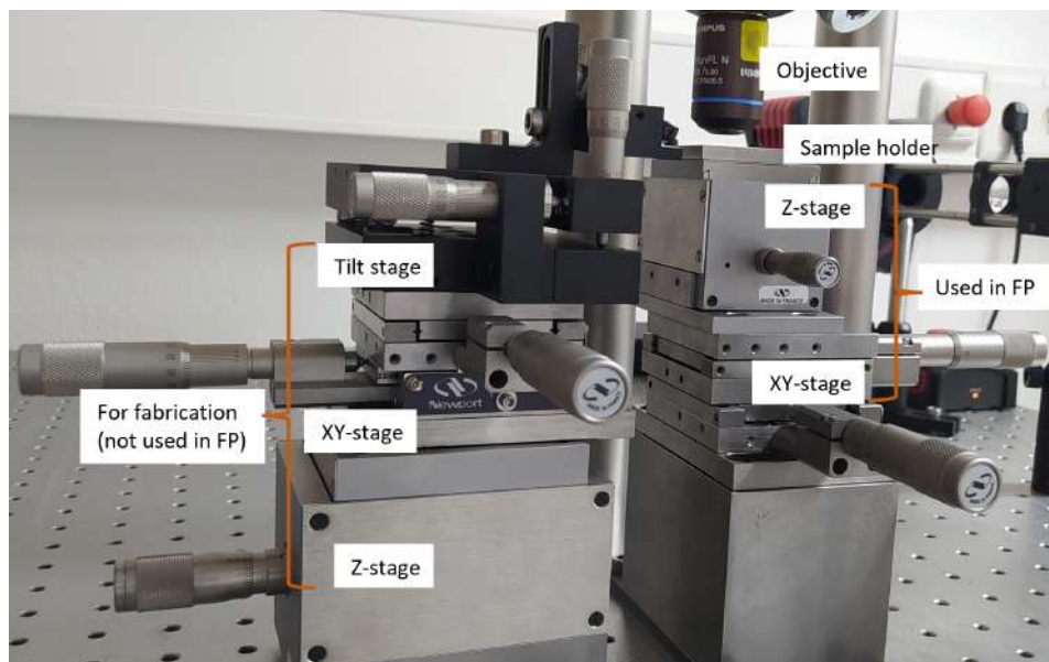
Figure 11: Two sets of manual stages are present in the set up for the placing samples and aligning them. Only the stack on the right side is used during the FP.
